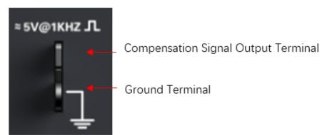
signal output terminal marked in the figure below.
