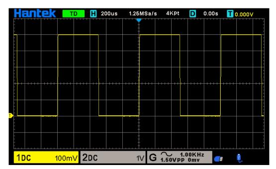
Check CH2 channels using the same method. If the square wave waveform displayed in the time base does not match the figure above, you can follow the instructions in the section on <a href="Probe Compensation">Probe Compensation</a>.
