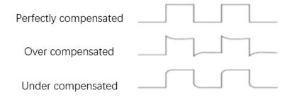
If necessary, use a non-metallic screwdriver to adjust the variable capacitance on the probe until the waveform displayed on the screen is "Perfectly compensated" as shown in the figure above. If necessary, repeat this step.
